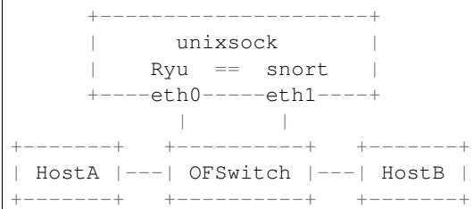
The above depicts Ryu and Snort architecture. Ryu receives Snort alert packet via **Unix Domain Socket**. To monitor packets between HostA and HostB, installing a flow that mirrors packets to Snort.
